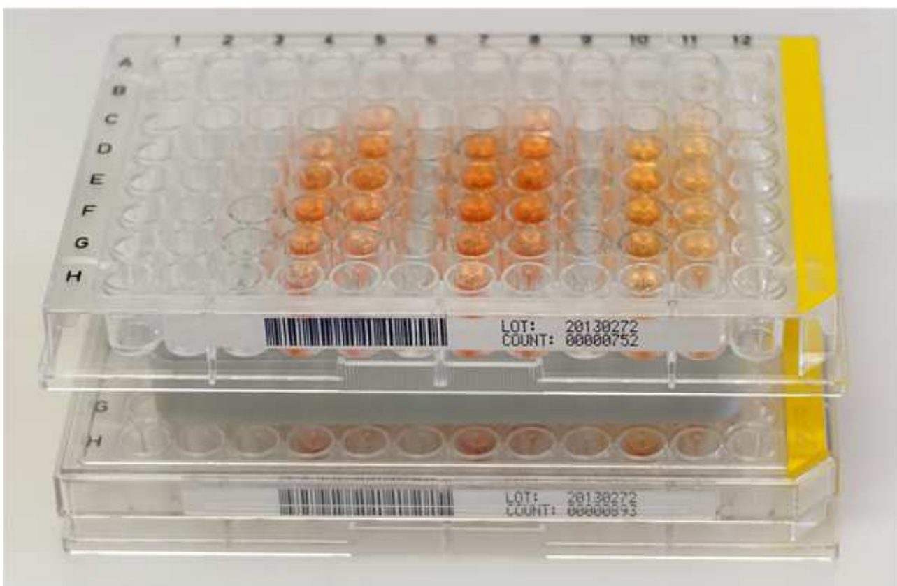
Figure 1: Alignment of 96-well plates below and above a Mini-Rayonex device with its lettering pointing upside and to the front. The multiplates were placed exactly in this way into the external incubator at 37.2 \pm 0.2 °C. The lower part of the figure represents the wells with seeded and exposed cells which have cleaved the tetrazolium dye due to their vitality and activity of mitochondrial dehydrogenases (orange coloured wells).
